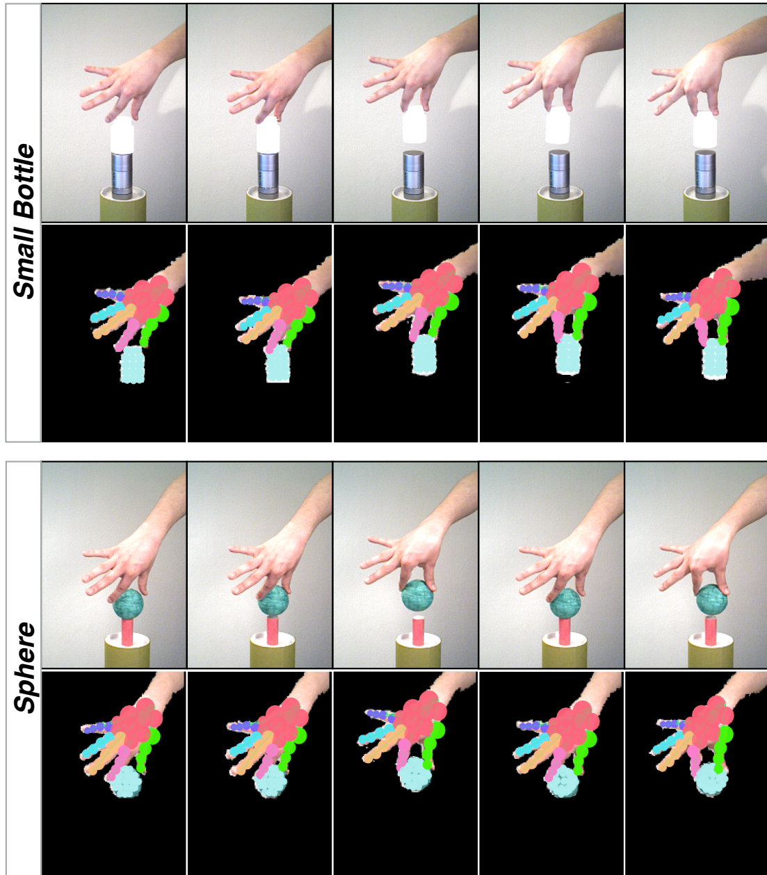
FIGURE 6.12: Qualitative results on the in-hand scanning sequences from Tzionas and Gall [3]. The top row shows color input frames and the bottom row tracking results in the Gaussian representation overlaid with the colored projection of the point cloud, respectively. Note that different grasps with thumb and index finger are accurately reconstructed by the tracker.
