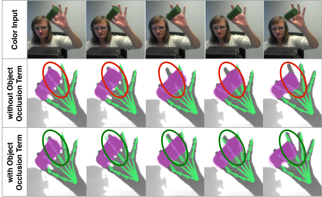
FIGURE 6.20: Comparison of the versions with Viewpoints (middle row) and with Object Terms with only E_o added (bottom row) on the Cylinder sequence. The color input (top row) is provided for reference and the tracking results are overlaid on the depth input. While the middle finger remains stable under occlusion when the object occlusion term is enabled, it moves implausibly without this term.
